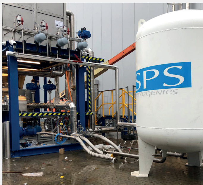
Figure 5: Side view of the demonstrator skid with thermal store (Dohmeyer & Frigologix).
